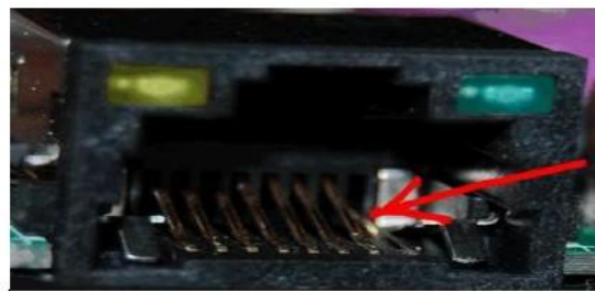
Ethernet Port Broken
