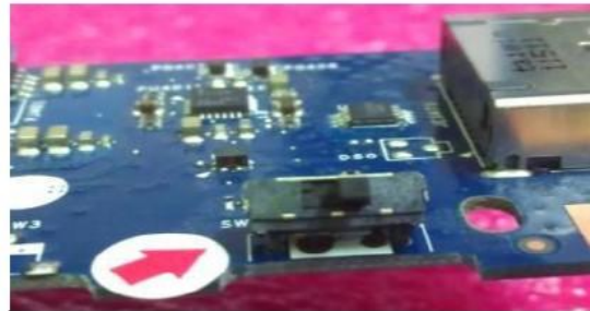
Wireless Switch Broken
