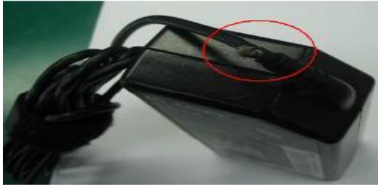
AC Adapter Cable Broken
