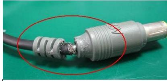
AC Adapter Cable Broken
