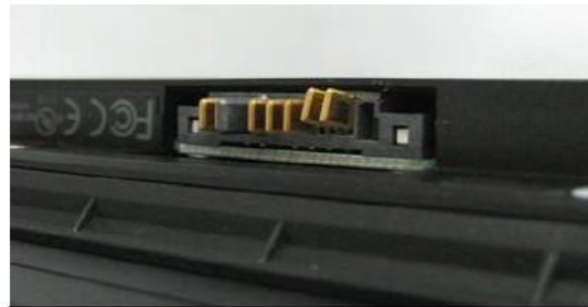
Battery Slot Broken
