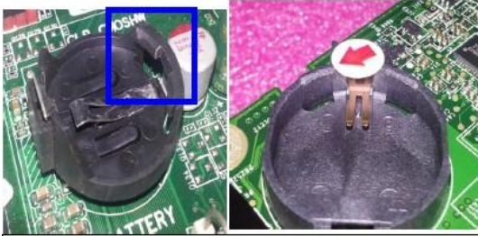
Battery Latch Broken Left: Good Right: Damaged
