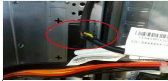
Internal Cable Broken
