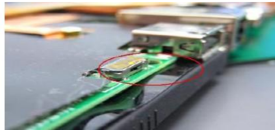
Wireless Switch Broken
