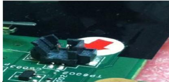
Damaged cable connector
